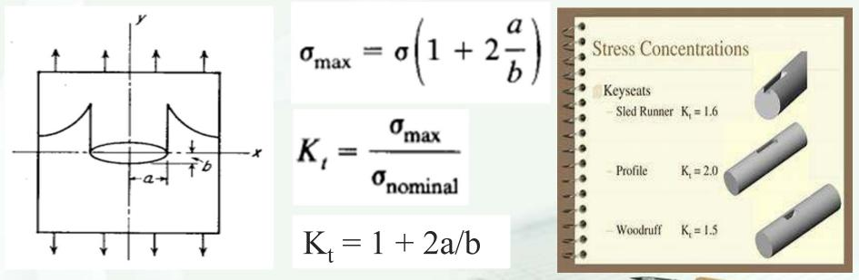
2a: Dimension of the hole perpendicular to the tension axis 2b: Dimension of the hole parallel to the stress axis For a circular hole, a = b, so  $K_t = 3$
